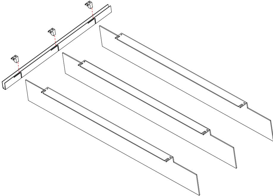
**2** With the black blocks inside the vertical profile, make it slide so the side of the shelves fit inside the slot.
