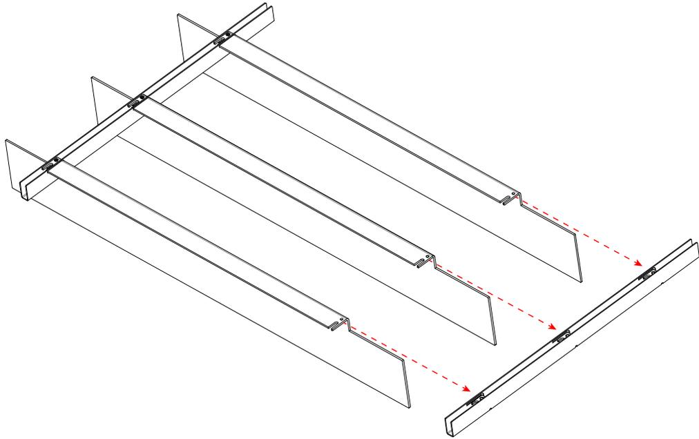
**8** Fix the block with the screw.
