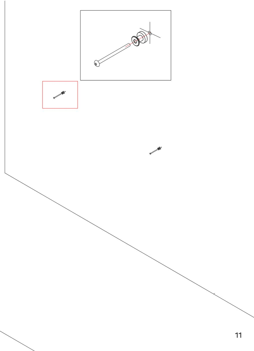
**11** Place the Wall shelves against the wall and make them slide downwards until they slide in the wall screws.
